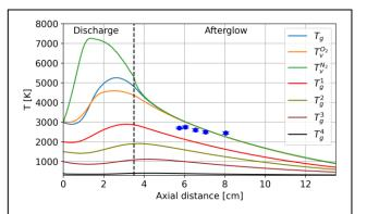
**Fig. 1**. Evolution of different temperatures as a function of axial distance.  $T_g$ ,  $T_v^{O_2}$  and  $T_v^{N_2}$  represent the gas temperature, vibrational temperatures of O<sub>2</sub> and N<sub>2</sub> in the center region of the tube.  $T_g^1$ ,  $T_g^2$ ,  $T_g^3$ ,  $T_g^4$  denote the gas temperatures of the four outer regions in the radial direction. Blue dots represent gas temperatures measured by Raman scattering in the afterglow [7].
